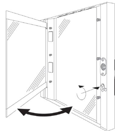
The door glass can be cleaned externally and internally. For this purpose, turn the stop holding the internal glass in position clockwise and, once the glass is opened, clean it with suitable detergent.
