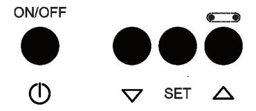
Key  $\bigcirc$   $\rightarrow$  Logical switch on/off of the control unit (passage from OFF status to functioning mode).
