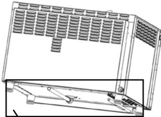
There is a sleeve (**A**) present in the lower part of the cooking chamber (in the centre) to which the bend and the rigid pipe supplied (**p**) must be connected. Couple the bend in the rigid pipe and connect it to the oven. Now, take the rigid pipe into the funnel (not provided).
