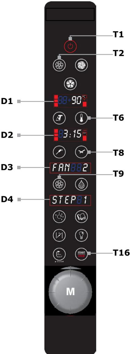
Once the oven has been switched on by pressing the **T1** key, select the convection cooking modality by pressing the **T2** key. Activate the desired cooking temperature set by pressing the **T6** key, signalled by the flashing of the key itself: set the temperature value by acting on the **M** knob (up to 280°C) and confirm the selection by pressing the **T6** key or the **M** knob of the encoder. The display automatically passes to the selection of the cooking time (the **T8** key flashes).
