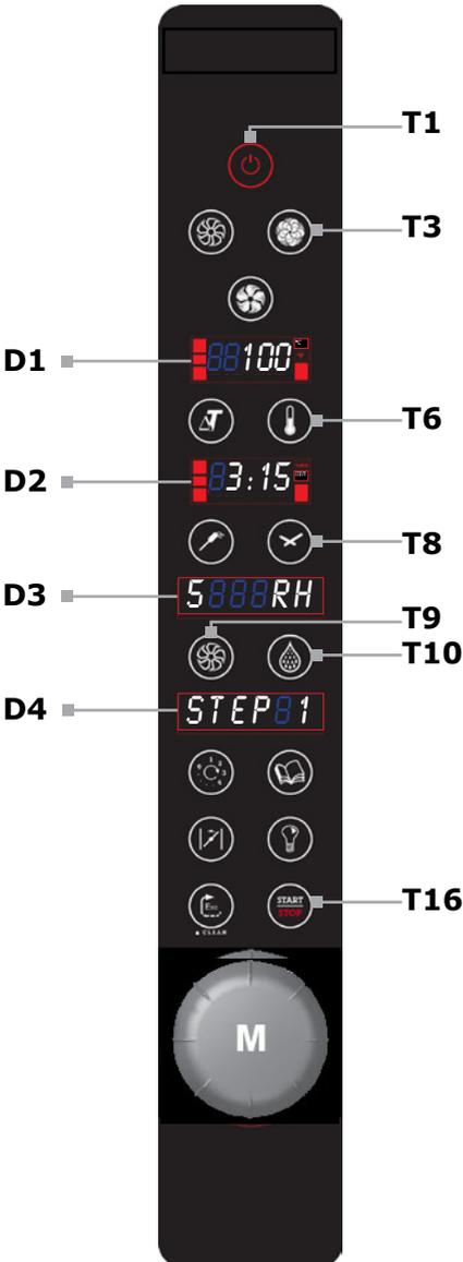
Once the oven has been switched on by pressing the **T1** key, select the steaming mode by pressing the **T3** key. Activate the desired cooking temperature setting by pressing the **T6** key, signalled by the flashing of the key itself: set the temperature value by acting on the **M** knob (up to 120°C) and confirm the selection by pressing the **T6** key or the **M** knob of the encoder.
