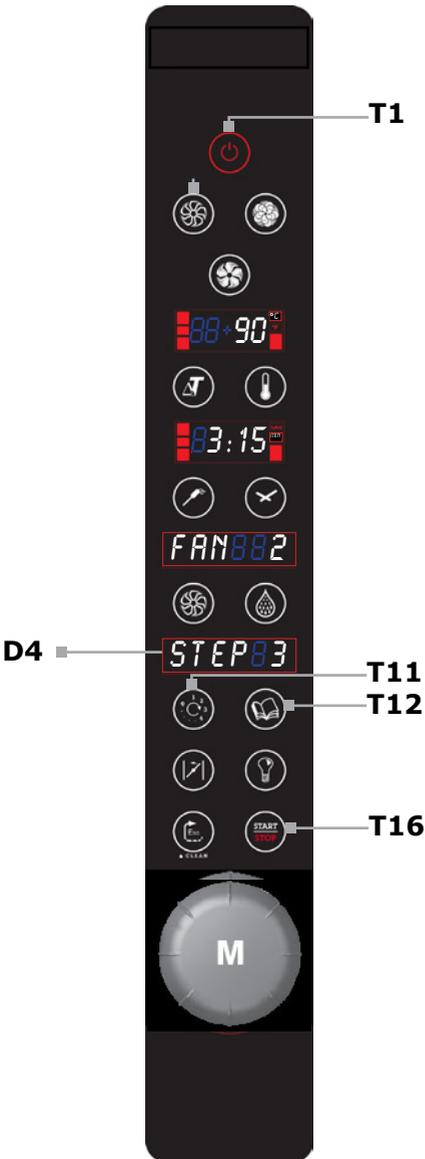
To access a memorised program, press the **T12** Book key and select the program number, shown on the **D4** display, by turning the **M** knob to right or to left. Confirm the selection by pressing the **M** knob when the desired program number is shown on the **D4** display. Ex.: **PRG804**
