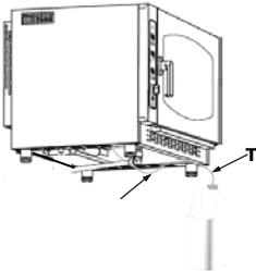
In the ovens with automatic washing, connect the small white/transparent plastic pipe (**T**) to the can of detergent, placing it as near to the bottom as possible.
