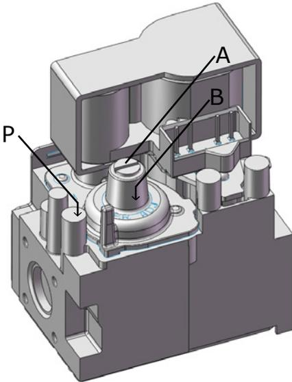
When the appliance is connected, turn it on and check the gas pressure.
