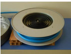
2) Assemble the hub and hook the central spring flap on the slot in the hub.
