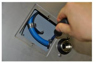
5) Wrap the hose onto the pulley (act on the hub of the spring with the 8 mm hex key if necessary).
