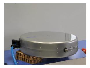
3) Remove the twelve side screws holding the shells together and unscrew the two pins, so as to have access to the internal components.
