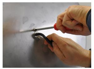
3) Loosen the hub gradually by turning the hex key counterclockwise, to fully unload the spring.
