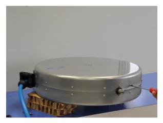
3) Reinsert the MaxiReel between the two holes of the wall bracket and its fixing pins.
