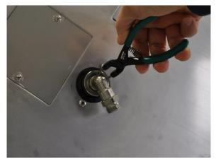
3) Connect the inlet flexible hose to the inlet unit  $M\frac{1}{2}$ "G of the MAXIReeI.
