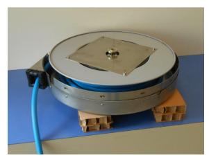
5) Take out the pulley assembly from the casing.
