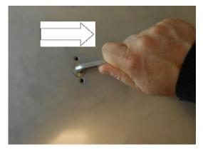
2) Hold the hex key firmly and tighten the two M4 screws holding the hub.
