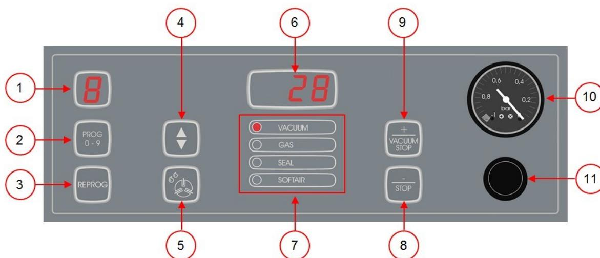
Figure 7: Control Panel of the 10-Program Control System
