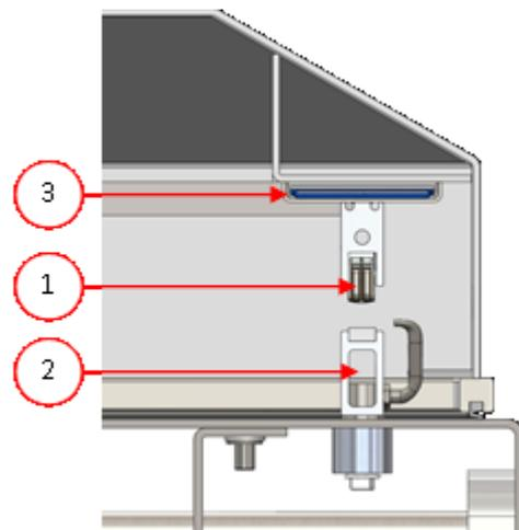
Figure 3: Overview of the Sealing System (Including Seal Bag)
