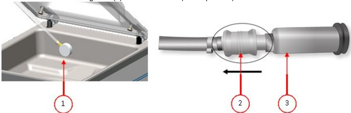
Figure 13: External Vacuum Adapter Set (1-Program Control)
