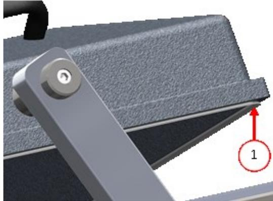
Figure 22: Replacing the Lid Gasket
