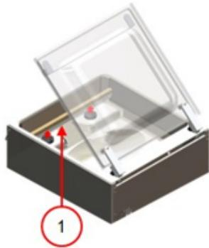
Figure 18: Removing the Sealing Bar (Plastic Lid)
