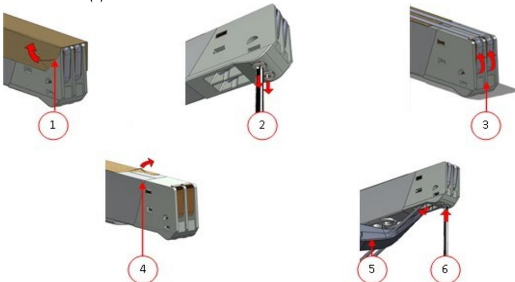
Figure 20: Replacing the Sealing Wire
