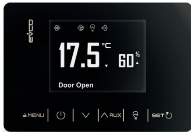
In order to store the chocolate, the temperature set point must be +12/+18 and humidity must be under %65 RH. Do not change the humidity and temperature values of refrigerator. All the needed processes are carried out in the factory to keep the humidity and temperature of the product in optimum values.
