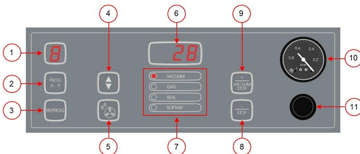
Figure 6: Control Panel of the 10-Program Control System
