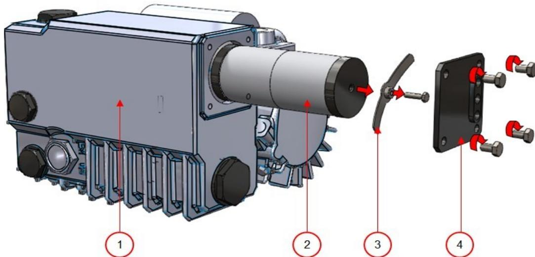
Figure 18: Replacing the Oil Exhaust Filter (Pump 16 m<sup>3</sup>)
