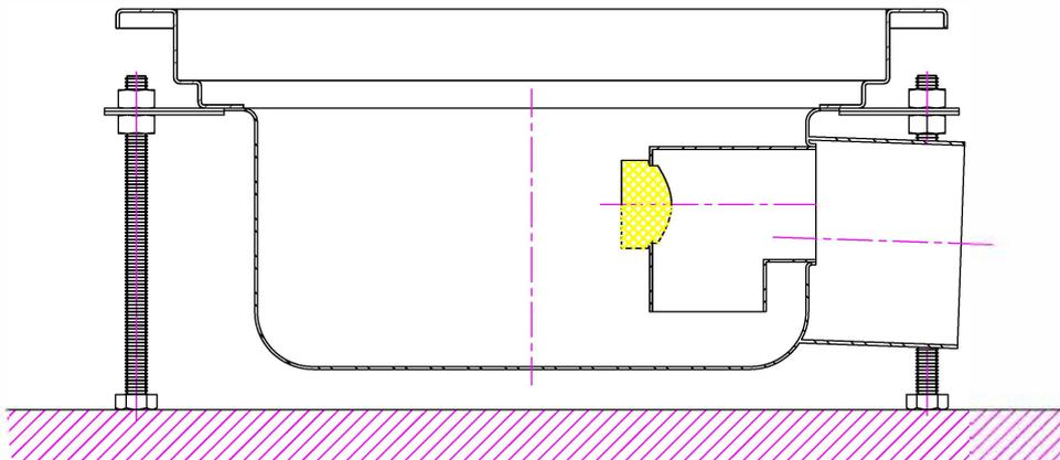
**\* THE DRAINAGE CHANNEL IS CONNECTED TO THE PVC PIPE. PLEASE MAKE SURE TO HAVE THE REQUIRED SLOPE AND THE ANGLE OF FLOW.**
