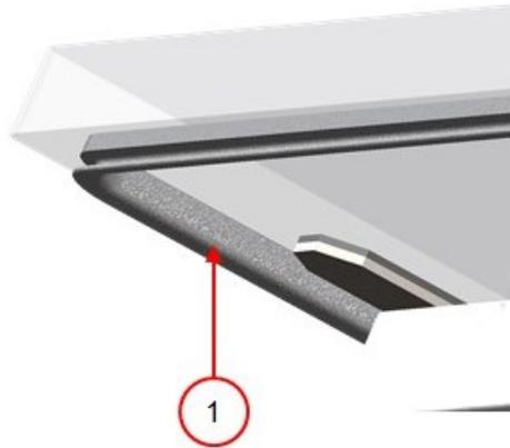
Figure 16: Replacing the Lid Gasket
